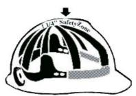
Hard hats require a hard outer shell and a shock-absorbing lining. The lining should incorporate a head band and straps that suspend the shell from 1 to 1 1/4 inches (2.54 cm to 3.18 cm) away from the user's head. This design provides shock absorption during impact and ventilation during wear.
